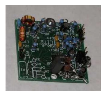
20 M board with ugly construction Xtal oscilator with x3 output [no coils, no tuning !]
