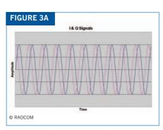
FIGURE 3A: I AND Q SIGNALS AT THE OUTPUT OF THE MIXERS.
