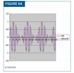
FIGURE 6A: AM I AND Q SIGNALS AT THE INPUT TO THE SOUND CARD.
