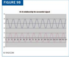
FIGURE 9B: I AND Q PHASE RELATIONSHIP FOR UNWANTED SIGNAL
