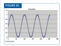
FIGURE 6B: SAMPLED I AND Q AM SIGNALS. FIGURE 6C: AM DEMODULATION USING I AND Q.
