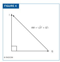
FIGURE 4: AM MODULATION USING I AND Q.
