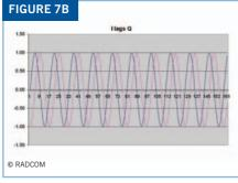
FIGURE 7B: UNWANTED SIGNAL I AND Q PHASE RELATIONSHIP.
