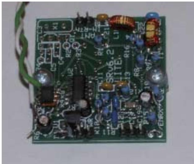
Xtal parts removed and DDS input to pin1 [.01uF Cap under ICS501] 18Mhz in & x3 output at 56MHz +
