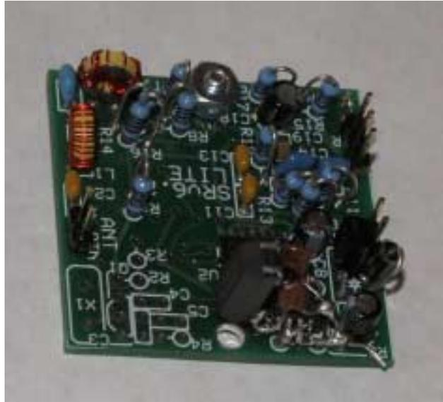
20 M board with ugly construction Xtal oscillator with x3 output [no coils, no tuning !]
